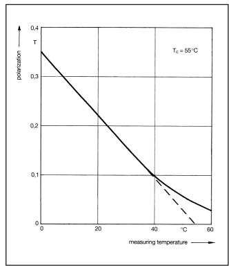
Fig. 12: Polarization Temperature Curve of THERMOFLUX 55/100 G
