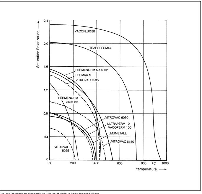
Fig. 10: Polarization Temperature Curves of Various Soft Magnetic Alloys.
