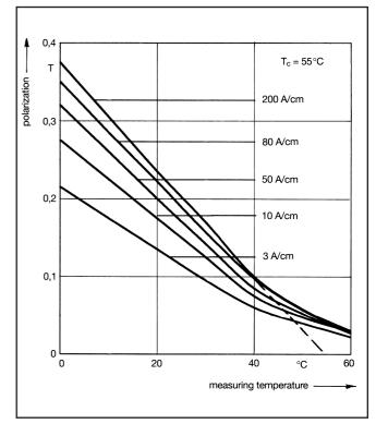
Fig. 13: Polarization Temperature Curves of THERMOFLUX 55/100 G as a Function of Field Strength (f = 50 Hz)
