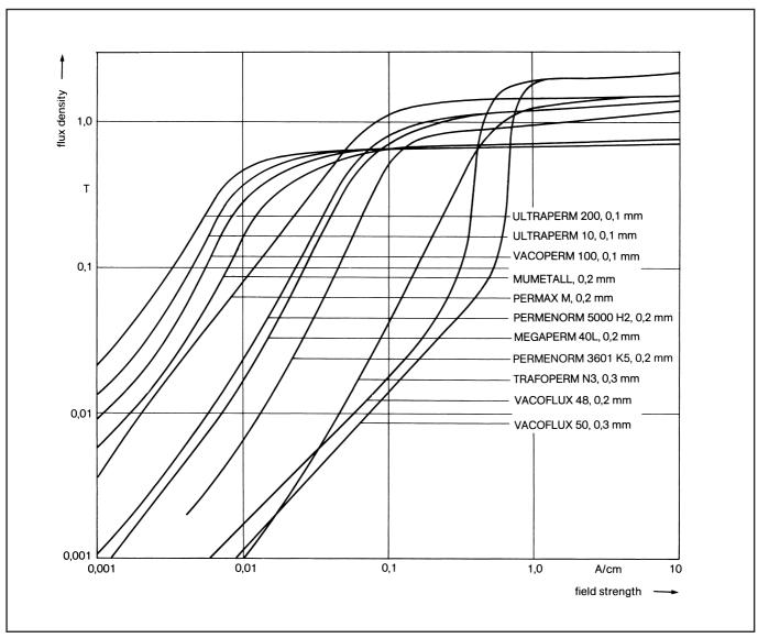
Fig. 8: Dynamic (50 Hz) Flux Density Field Strength Curves of Strips, Strip Thickness: ≤0.3 mm. Measured on Toroidal Cores
