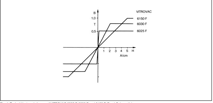
Fig. 4: Typical Hysteresis Loops of VITROVAC 6025 F, 6030 F and 6150 F (Semi-Schematic)
