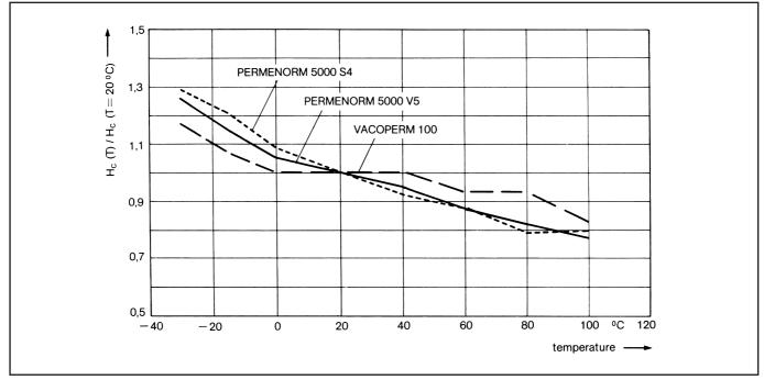
Fig. 11: Relative Temperature Dependency of Coercivity H<sub>c</sub> (Standardized to 20°C) of PERMENORM 5000 V5, PERMENORM 5000 S4 and VACOPERM 100.
