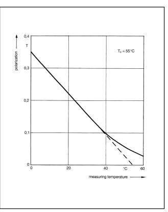
Fig. 3: Polarization Temperature Curve of THERMOFLUX 55/100-G.
