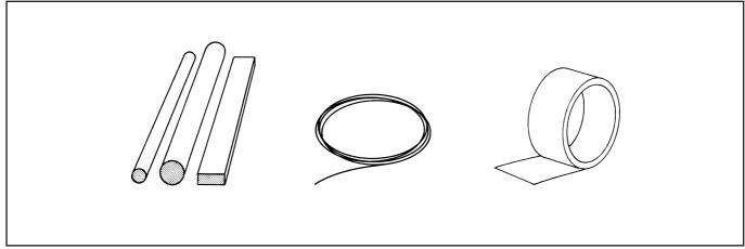
Fig. 5: Different Forms of Semi-finished Products
