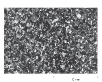
Fine Grained Microstructure of PERMENORM 5000 V5
